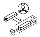
Replaceable control gear by a professional.
